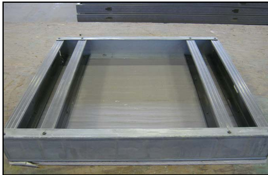
Figure 1: Test Specimen Frame (Typical)
