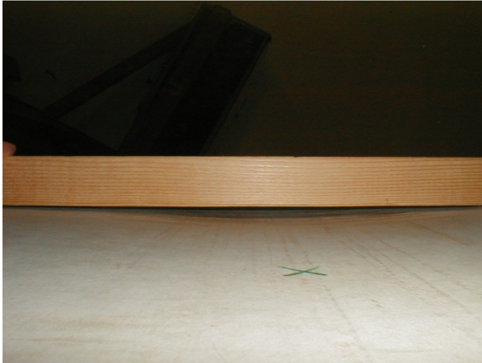
Photo 2: Indentation of panel at point of impact for the first test. The wooden slat being held across the panel is 1.5 inches tall.
