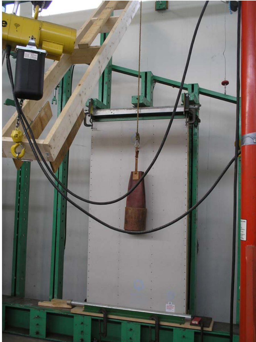
Photo 1: General test set-up for specimen vertical impact testing. As shown, bag is set to impact on panel face between studs.
