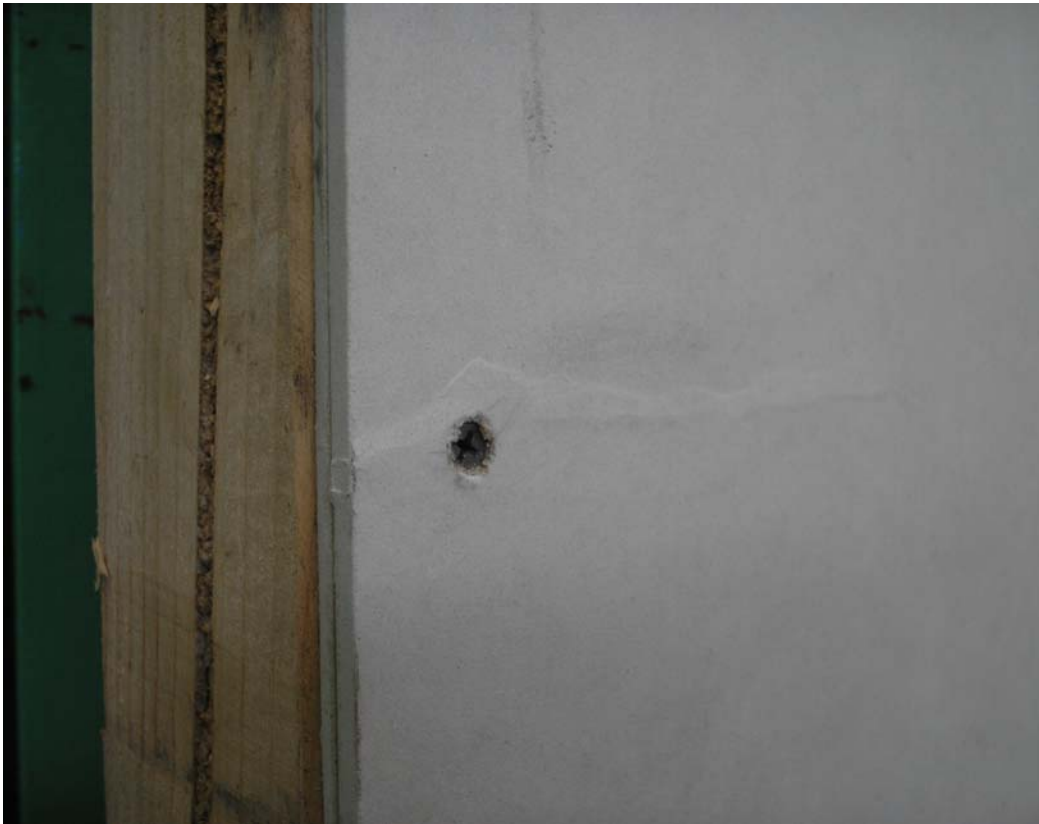
Photo 4: “Kinking” of the panel face during test three.
