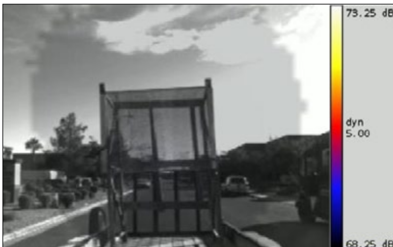
Figure 2: SoundCam Results - Treated Panel (2 Coats of QuietCoat®)
