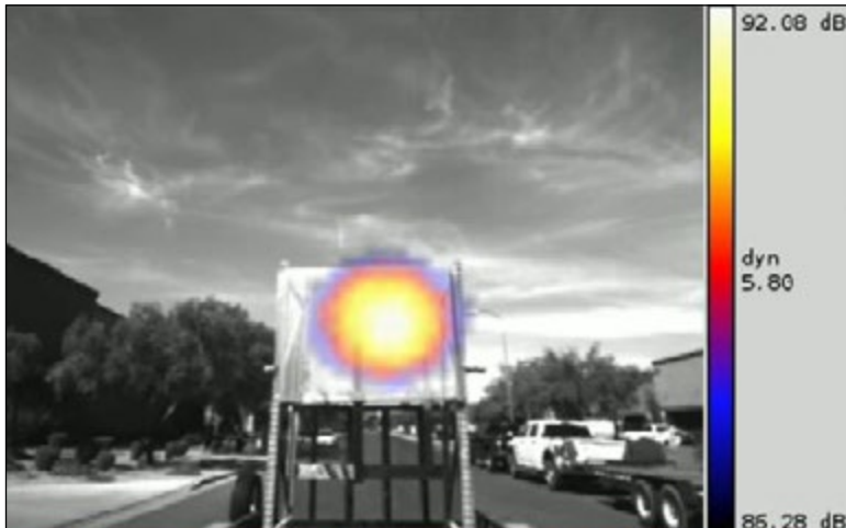
Figure 2: SoundCam Results - Treated Panel (2 Coats of QuietCoat®)
